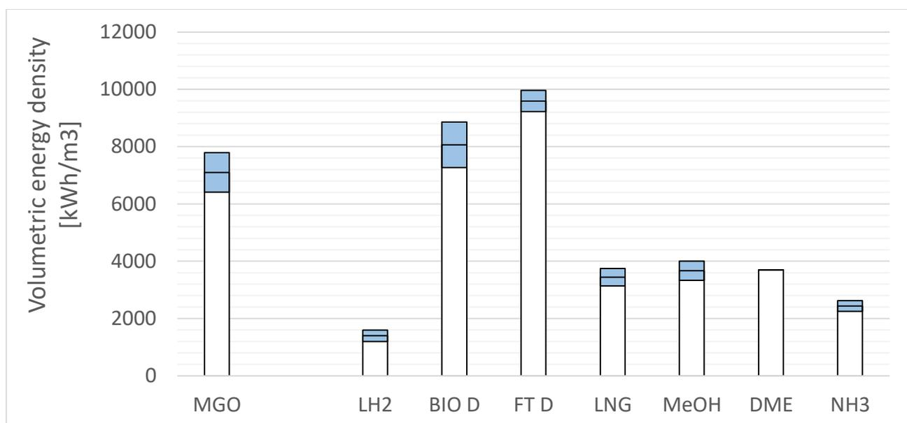
**Figure 2: Volumetric energy density of future fuels including the storage system of the concerned fuel. The benchmark (MGO) has been compensated for the efficiency difference between diesel generators (43%) and SOFC (55%). The blue bars show the data ranges found in literature, projects, and supplier specifications. Based on LHV of fuels. (Aceves et al., 2010; Sapra, 2020; van Biert et al., 2016; van Veldhuizen et al., 2020)**
