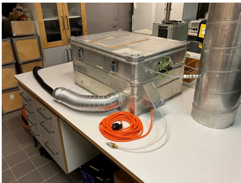
Figure 4: Weatherproof box for exhaust extraction
