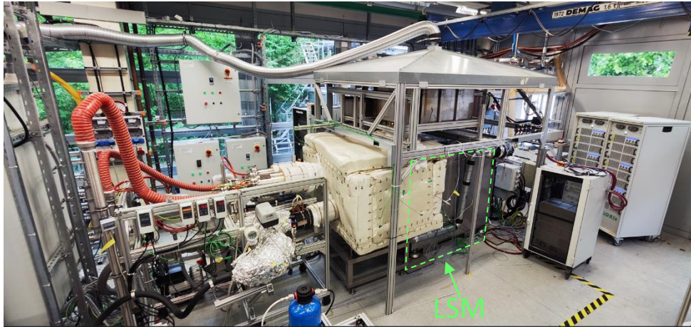
Figure 2 GALACTICA test rig with 30 kWe LSM from SolydEra
